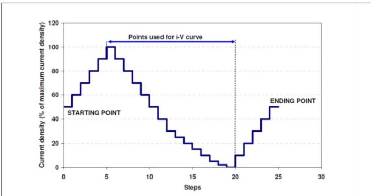
Figure 1: Example of current density cycle with 25 steps of instantaneous change in current density. In this example, the starting and ending points of this profile are chosen to be at 50% of the maximum current density.
