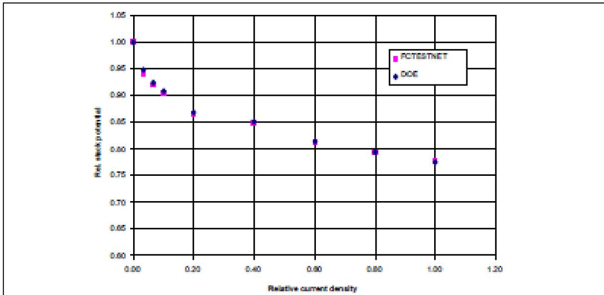
Figure 3 : Example polarisation curve recorded using DOE and FCTES<sup>QA</sup> procedures on 15 kW stack [1].
