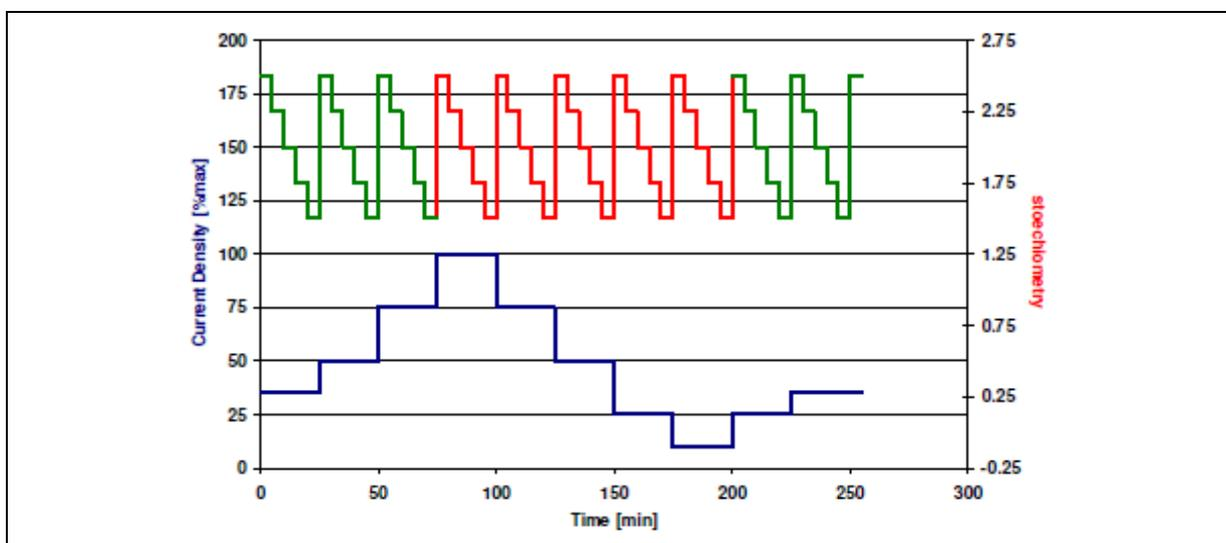
Figure 4: Example of one complete current density with 5 set points  $k$  and stoichiometry cycles of the 5 reactant stoichiometry values  $h$  at each set point.
