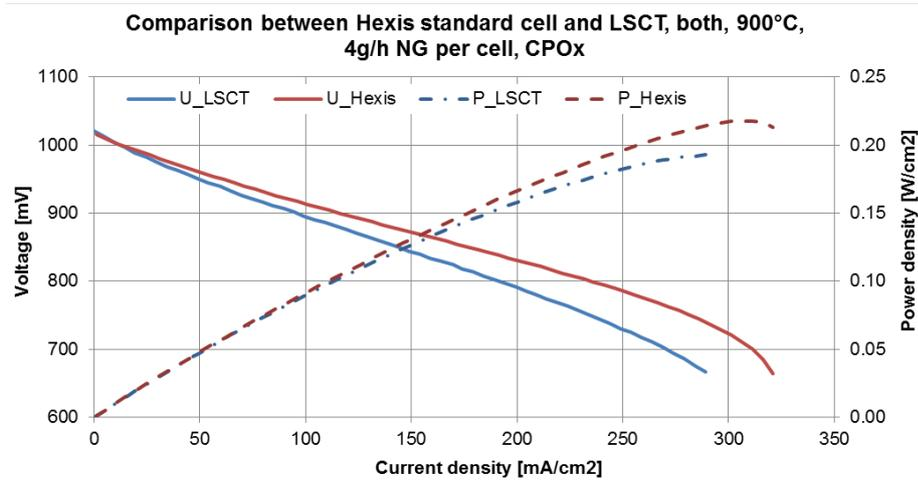
**Figure 4:** IV and performance characteristic of the cell with the LSCT anode in comparison with the Hexis cell (start of experiment). A fuel utilisation of 80% is reached around 250 mA/cm<sup>2</sup>.
