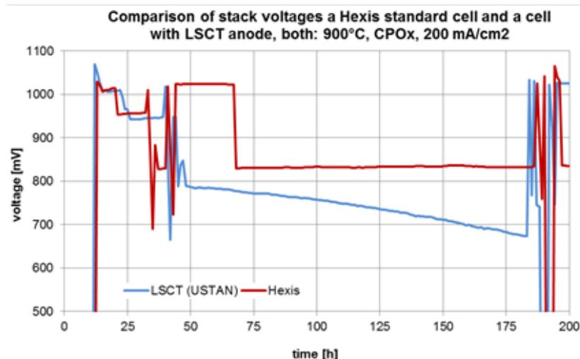
**Figure 5:** Comparison of the stack potential over time between cells with the LSCT anodes and Hexis standard cells
