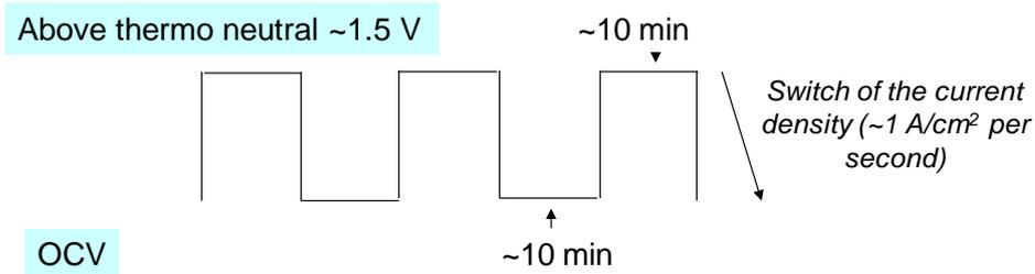
Figure 1: Cell voltages cycling from OCV to either thermo neutral, or exothermal mode of operation with two duration plateaus, i.e. 30 seconds and 10 minutes.
