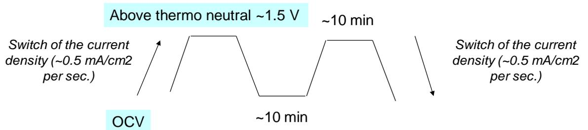
Figure 3: Cell voltages cycling from OCV to either thermo neutral, or exothermal mode of operation with a duration plateau of 10 minutes at each voltage. Speed for switching the current density is  $0.5 \text{ mA/cm}^2$  per second.
